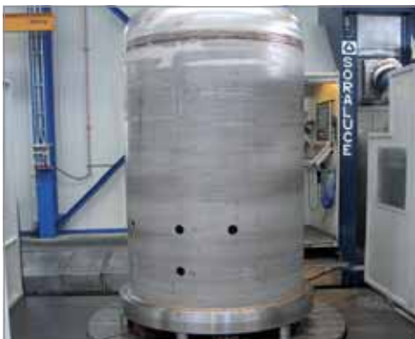
Turning and milling in one setting Rotary/ Turning Table DRCT 2500 / Ø 2500 / 20t
