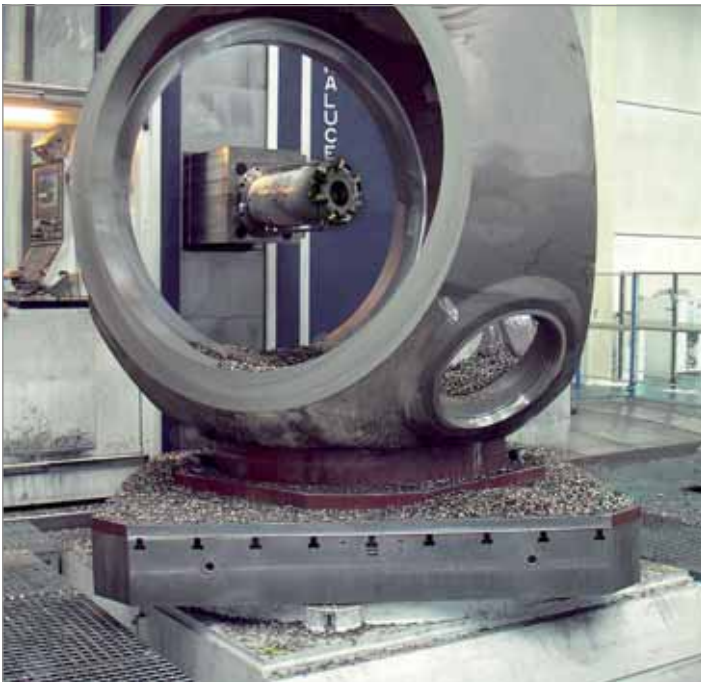
Tilt Tables for highly efficient nave manufacture DRLT 2500 / 2500x2500 / 2000 / 60t \pm 5^\circ
