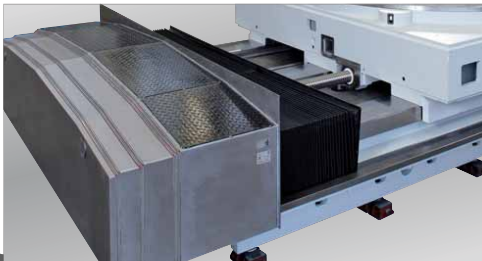
Reliable hydrostatics protection from dirt and emulsion through two separate covers.
