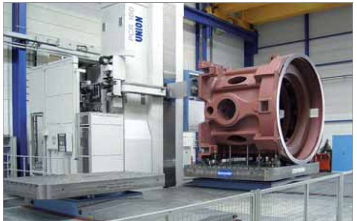
Manufacture of gearbox housings, Workpiece weight 100t DRLTS 3000 / 4000x3500 / 130t
