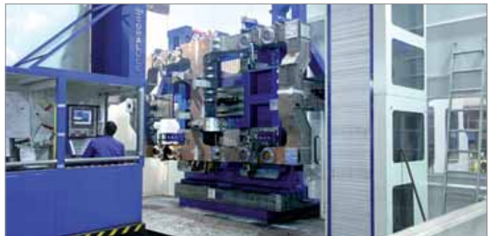
State-of-the-art manufacturing of pivot mounting Weight of fixture 20t, workpieces each 10t, DRTS 2500 / 3000x2500 / 60t
